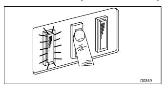
2. The yellow "HEATING ON" indicator light indicates that the heater is operating.
